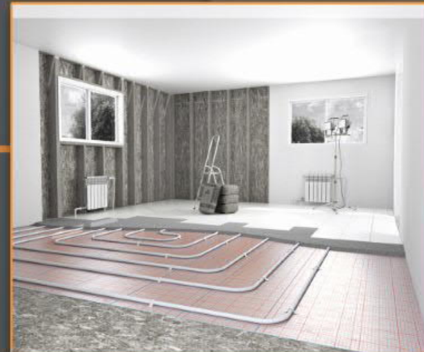
Under Floor Heating
